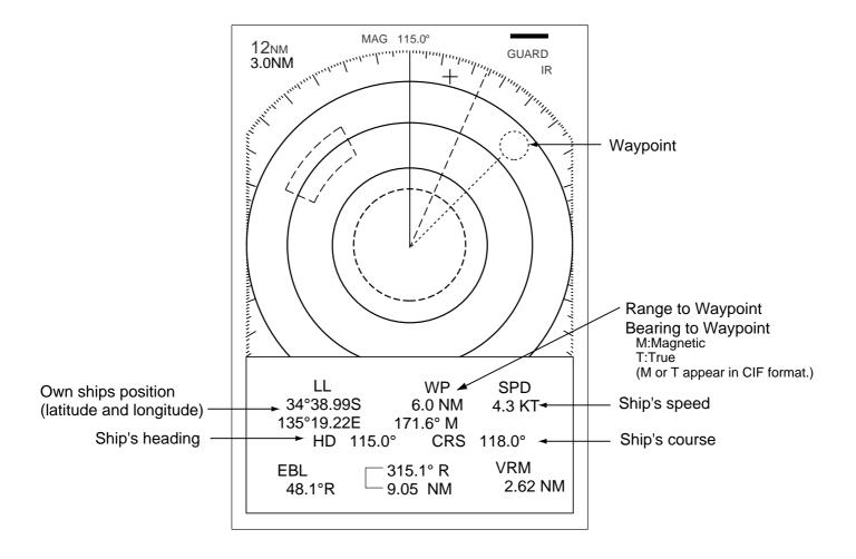
Figure 2-15 Navigation Data on the Screen
